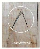
"With manual patching, there're always going to be defects on the edge of the patch, but with butterfly type patches, the patch is secure since the patch holds firmly and doesn't pop off later in the production process," Shawn Cheo states.
