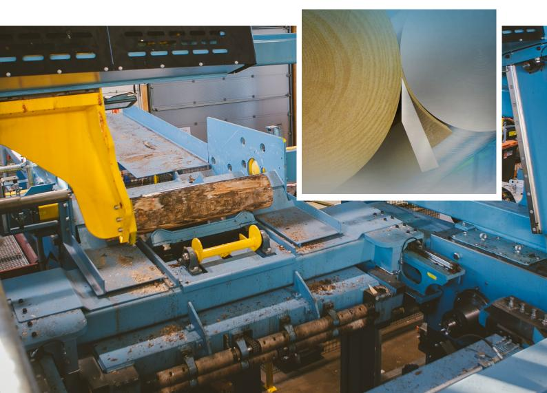
the Veneer Peeling Line R7-Hybrid Series. At each phase of the production process — centering, peeling, clipping, and grading — automation provides value. According to Mikko, these analyzers and processes can help you "boost your rate of full sheet recovery by as much as 15%."
