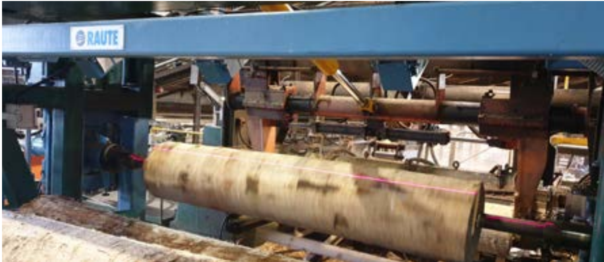
Block Centering Analyzer R7 - Peeling lasers ensure centering accuracy.
