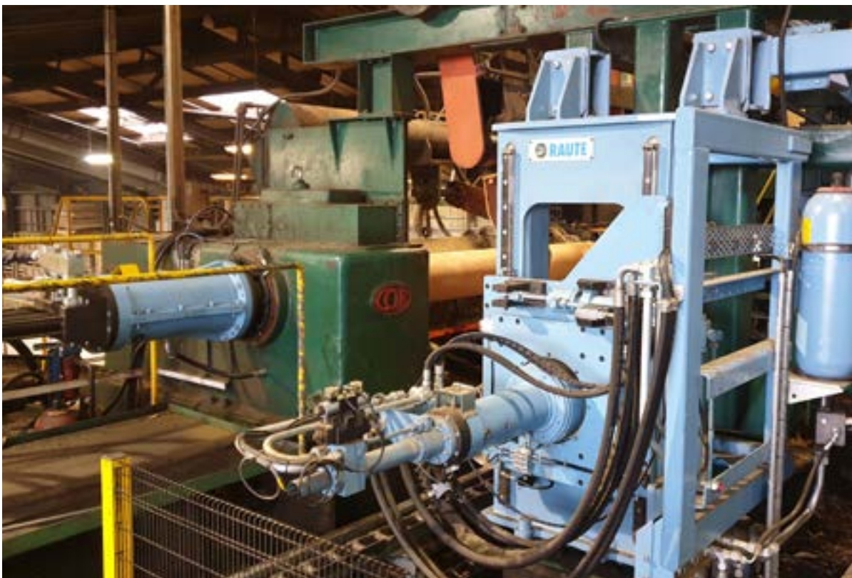
The new Raute XY-optimization unit installed in front of the COE (today part of USNR) lathe.
