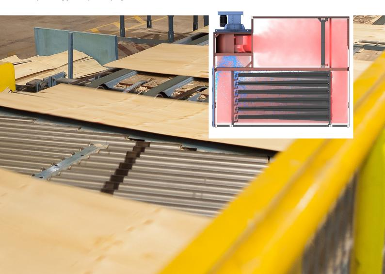
increased capacity without sacrificing efficiency. In contrast, conventional longitudinal drying technology handles airflow differently, making it more difficult to achieve a uniform application of the thermal mass, lower energy consumption, and reductions in the overall volume of dryer exhaust.
